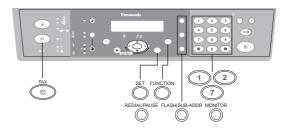
Make sure that the FAX Mode indicator is ON. If not, press FAX to select the "FAX MODE".
