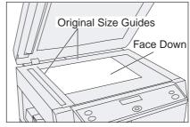
Place a book or an original Face Down on the Platen Glass, aligning it with the arrow mark on the Original Size Guides.
