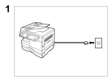
Unplug the Telephone Line Cable from the telephone jack that was supplied by the telephone company.
