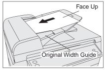
Place the original(s) Face Up on the ADF until the leading edge placed into the machine stops. Adjust the Original Width Guides to center the original(s) on the ADF.
