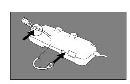
Turn the Power Switch OFF when installing the handset kit. Remove the handset kit out of the carton. Connect the handset cord to the handset cradle.
