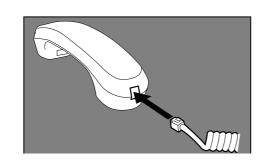
Connect the handset cord into the receiver. Place the receiver on the cradle. Turn the Power Switch ON.
