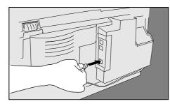
Connect the cable from the handset cradle into the HANDSET jack on the rear of the machine.
