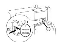
(5) Install a New Lithium Battery into the battery holder.
