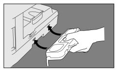
Hook the projections of the handset cradle into square holes on the left side of the machine.
